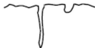
(h) Pores and cracks
